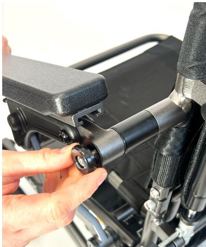
6. Put the armrest back in place and secure it with the central bolt onto the backrest.
