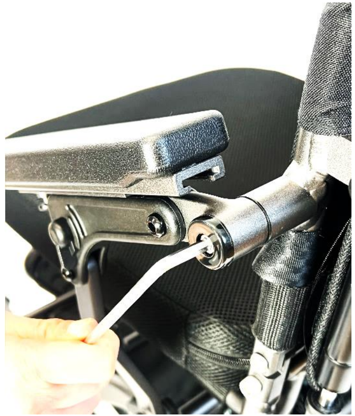
2. Remove the upper armrest mount by unscrewing the central bolt and remove the armrest.
