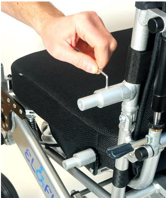
3. Securely tighten the small hex screws that will hold the spacers in place.
