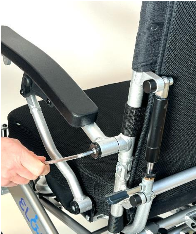
1. Remove the armrest by unscrewing the the upper and lower bolt with a hex wrench (Allen key).
