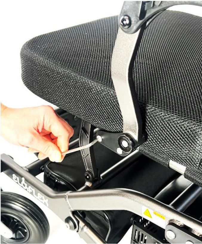
1. Remove the two bolts holding the lower bracket plate with a hex wrench (Allen key).
