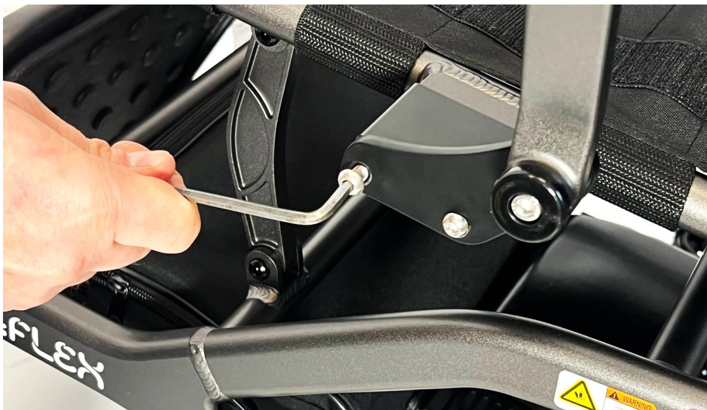
7. Secure the seat spacer and bracket with the 2 longer bolts onto the seat chassis.
