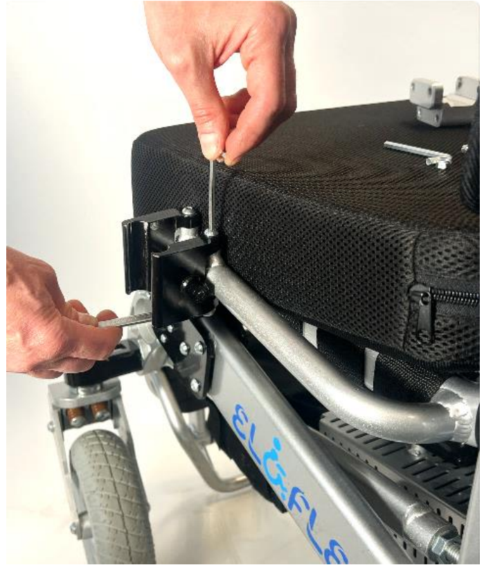
2. Undo the bolts holding the armrest clamp using a ring spanner and a hex wrench (Allen key) and remove the clamp.
