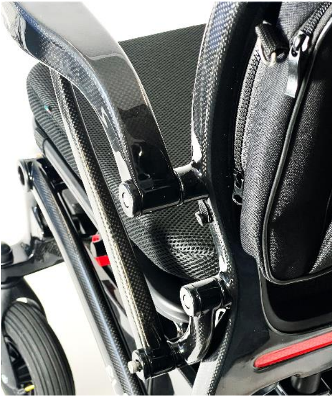
1. Remove the armrest by unscrew the central bolt with a hex wrench (Allen key).
