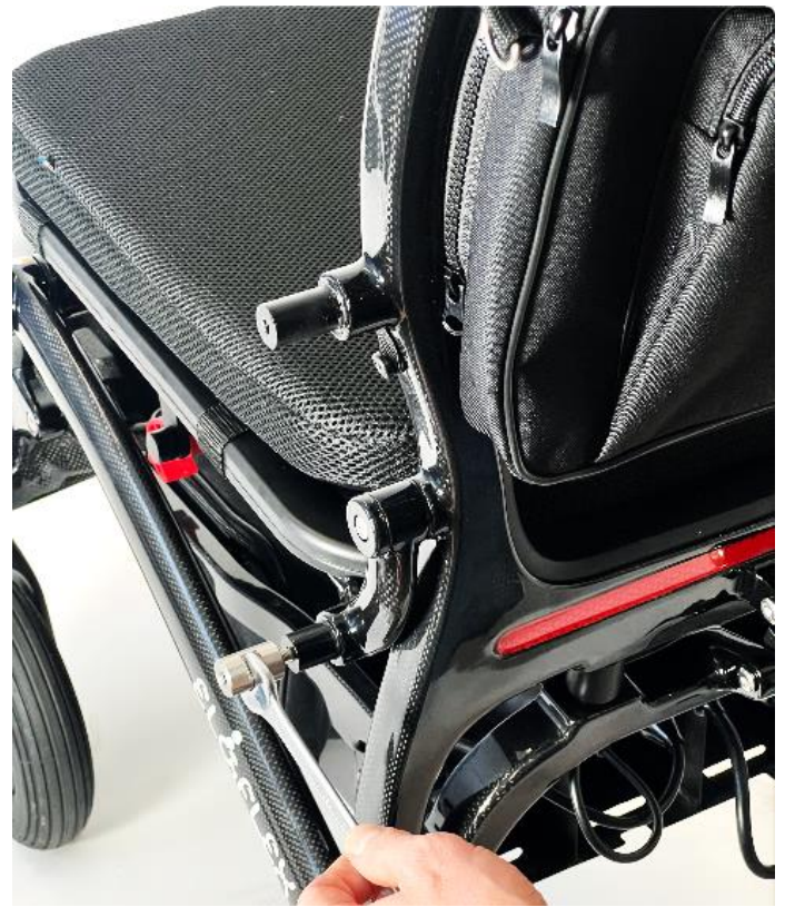
2. Mount the 4 pcs inner tap spacers onto the chassis, securing them tightly with an open-ended spanner (wrench).
